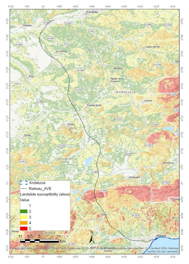
Figure 51: Different levels of landslide susceptibility and location of the railway track (case study 2a). (Source: ELSUS v2, Wilde et al., 2018)
