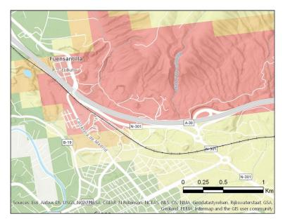
Figure 52: Detail of the railway tracks exposed at high and very high risk of landslide for the case study 2b, Murcia region. (Source: ELSUS v2, Wilde et al., 2018)
