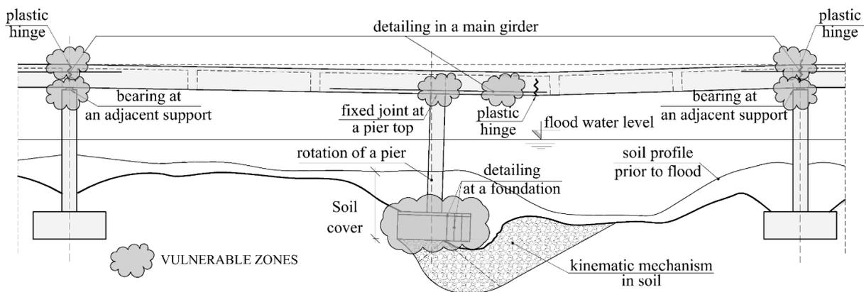
**Figure 16:** An example of a failure mode due to local scour at a pier - multiple-span RC girder bridge and its vulnerable zones - adapted from Tanasic & Hajdin, 2017
