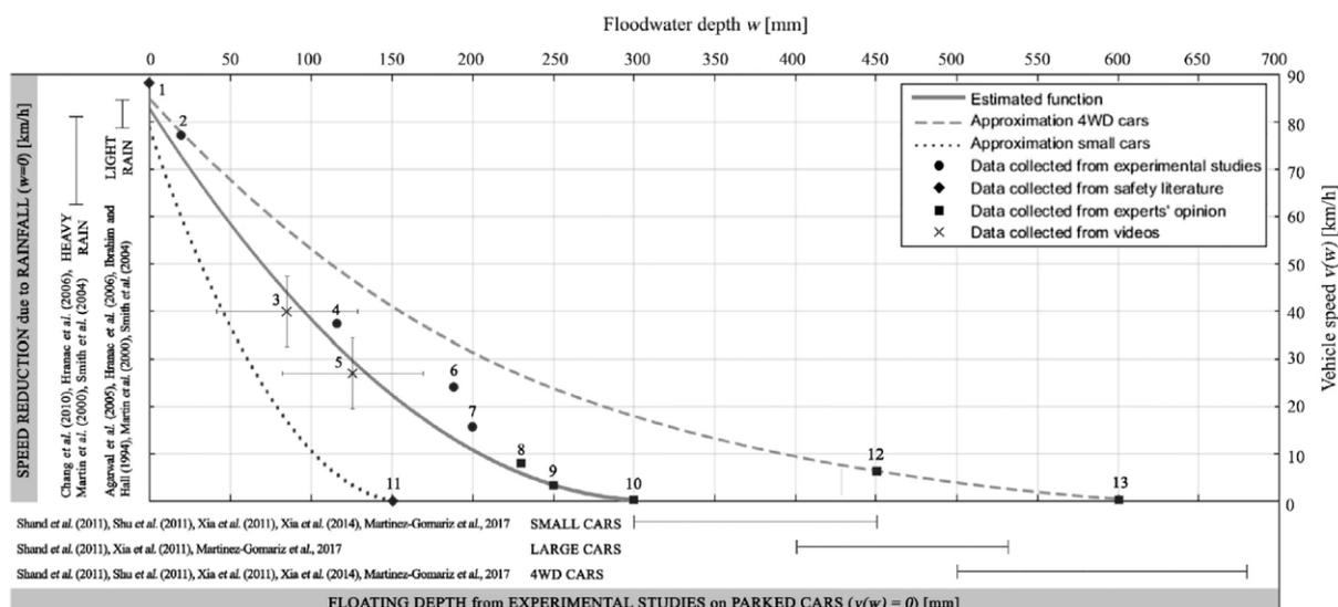
**Figure 12:** Depth-disruption function relating flood depth on a road with vehicle speed (Pregnolato et al. 2017)
