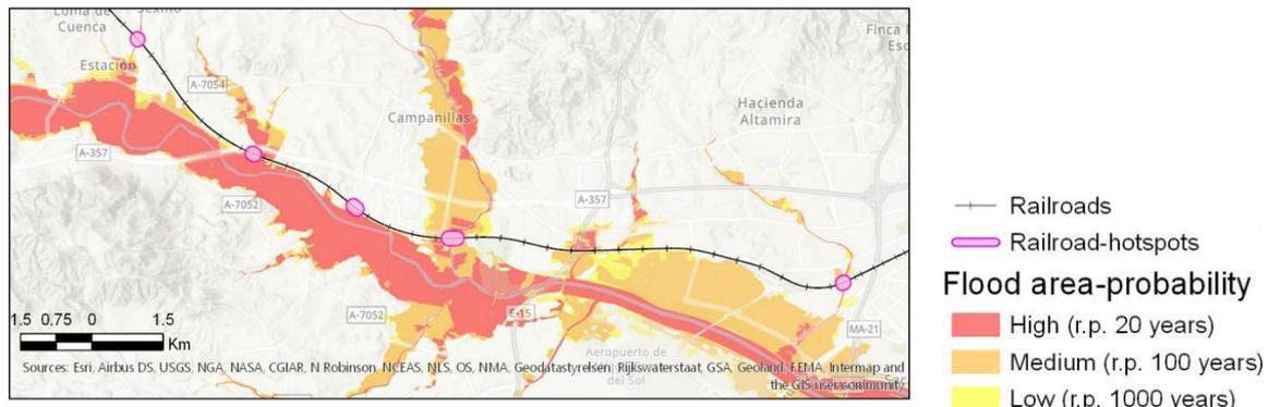
**Figure 20:** Exposure of railway track to floods for different flood return periods (20-years, 100-years and 1000-years). The exposed parts of the railway are indicated with pink ellipses. (Source: *Ministerio para la Transición Ecológica*, <https://www.miteco.gob.es/es/agua/temas/gestion-de-los-riesgos-de-inundacion/mapa-peligrosidad-riesgo-inundacion/>)
