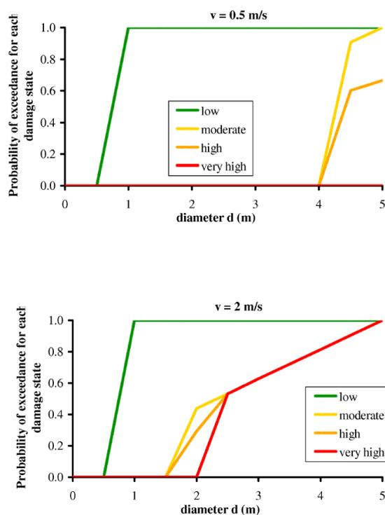
**Figure 10:** Fragility functions, expressing probability of exceeding damage states as a function of rock diameter for different rock velocities (Mavrouli and Corominas; 2010)
