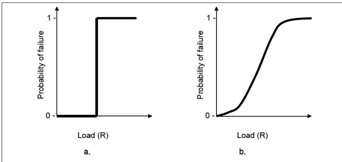
**Figure 6:** A conceptual fragility curve: (a) step function for very well understood or brittle systems; (b) an S-shaped function for poorly understood or elastic systems (USACE, 2010)
