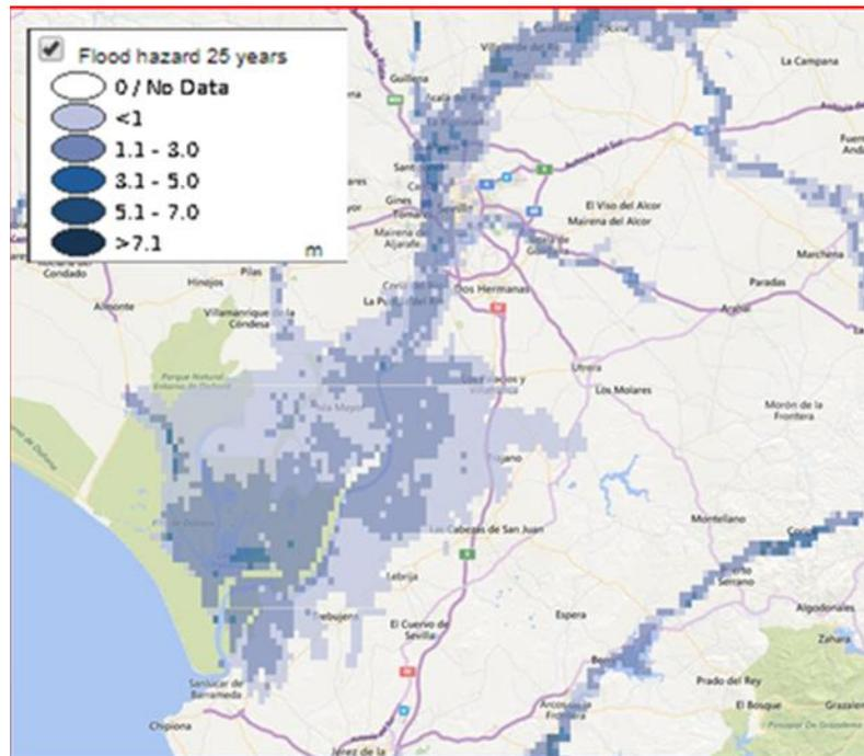
**Figure 19:** Flood depth for flood with return period 25 years. (Source: Global Assessment Report on Disaster Risk Reduction)
