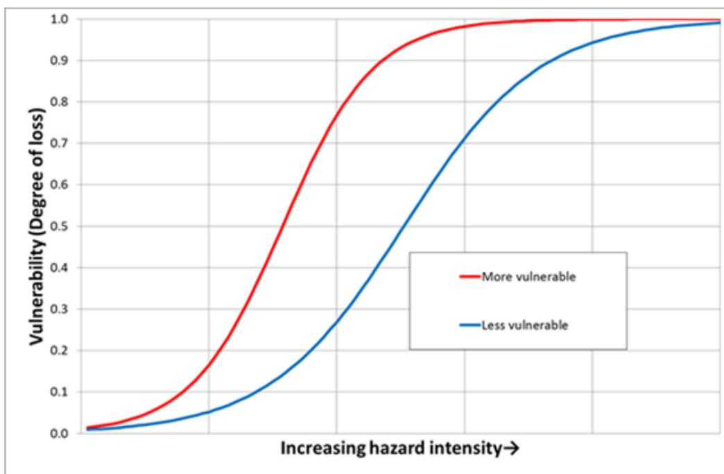
**Figure 7:** General function expressing the degree of loss as a function of hazard intensity
