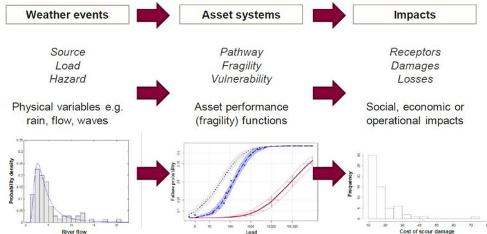
**Figure 2:** Conceptual risk model (Lamb et al.; 2017). The lower figure row applies to bridge failure from scour
