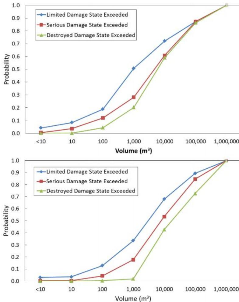
**Figure 14:** Fragility curves for roads hit by debris flow. Top: Local (low-speed) roads. Bottom: High speed roads. The volume on the horizontal scale refer to the volume of debris intersecting the road
