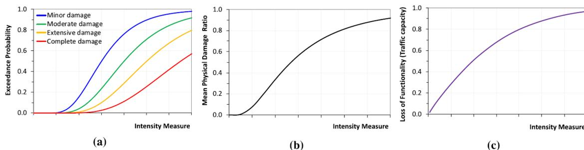
**Figure 5:** Example of fragility functions (a), degree-of-loss functions (b) and functionality loss functions (c), as the function of a hazard intensity
