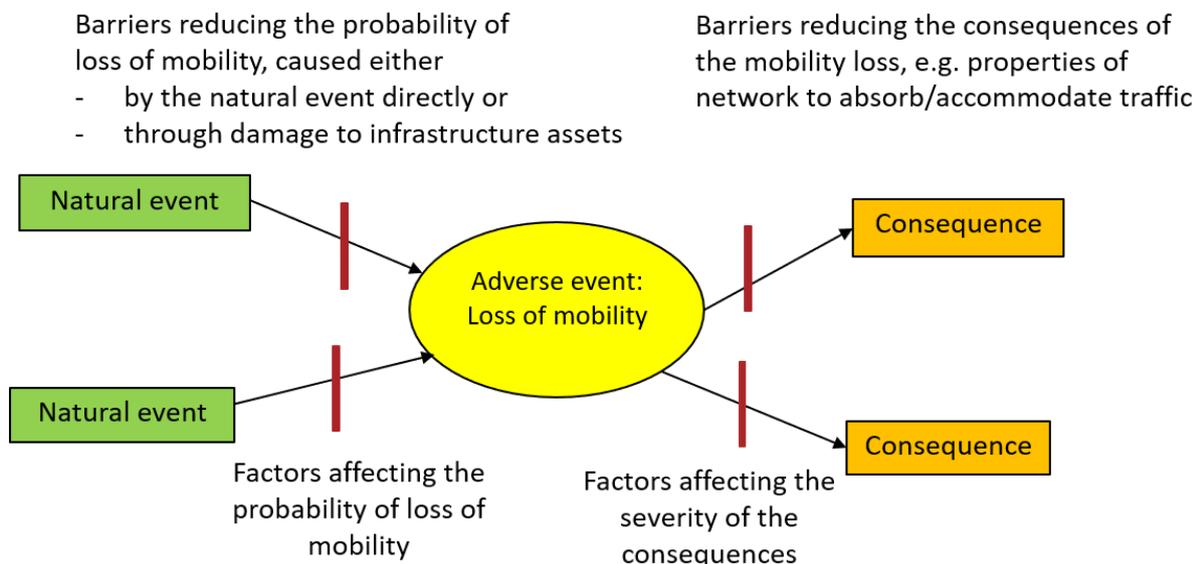
**Figure 1:** Schematic bow-tie representation of the scope of the work
