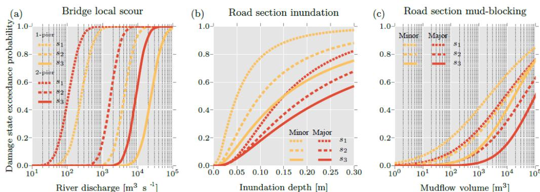
**Figure 13:** Functional loss functions for (a) bridge local scour, (b) road section inundation, and (c) road section mud-blocking. The horizontal axis represents the intensity measure 4 of the corresponding hazard. For (a) bridge local scour and (c) road section mud blocking the axes are displayed in log-scale. The vertical axis represents the expected functional loss (Hackl et al.;2018)
