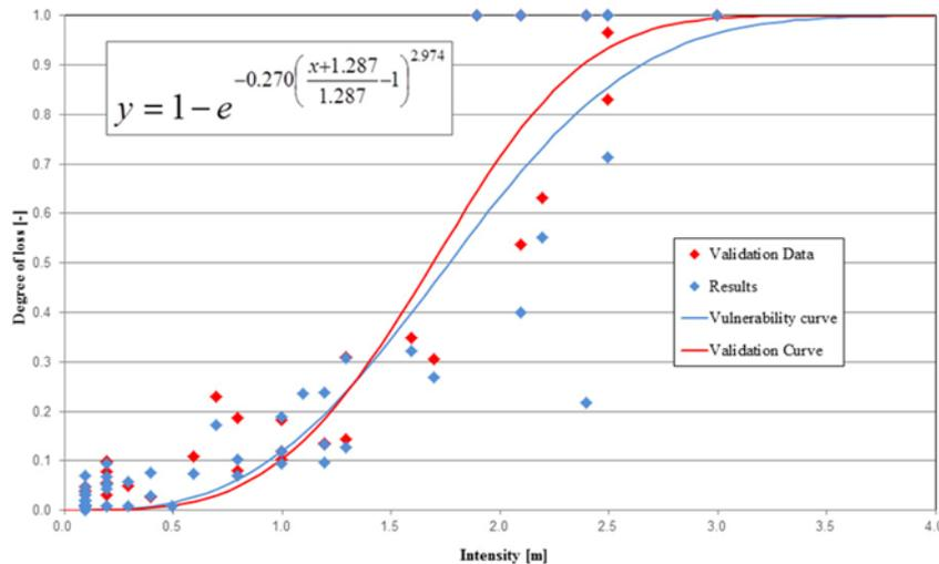
**Figure 8:** Development of a structural vulnerability function from empirical data for buildings hit by debris flow. The function expresses the degree of loss as a function of debris height in m. (Papathoma-Köhle et al. 2012)
