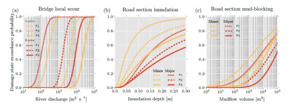
**Figure 13:** Functional loss functions for (a) bridge local scour, (b) road section inundation, and (c) road section mud-blocking. The horizontal axis represents the intensity measure 4 of the corresponding hazard. For (a) bridge local scour and (c) road section mud blocking the axes are displayed in log-scale. The vertical axis represents the expected functional loss (Hackl et al.;2018)
