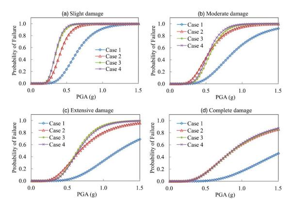
Figure 11: Comparison between the analytical and Bayesian updated fragility functions: (a) slight damage; (b) moderate damage; (c) extensive damage; (d) complete damage. Case 3: Bayesian updated curves of Case1 using hybrid simulation data; and Case 4: Bayesian updated curves of Case 2 using hybrid simulation data. (Singhal and Kiremidjian; 1998)
