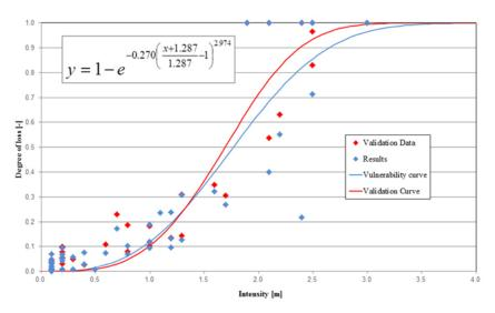
**Figure 8:** Development of a structural vulnerability function from empirical data for buildings hit by debris flow. The function expresses the degree of loss as a function of debris height in m. (Papathoma-Köhle et al. 2012)
