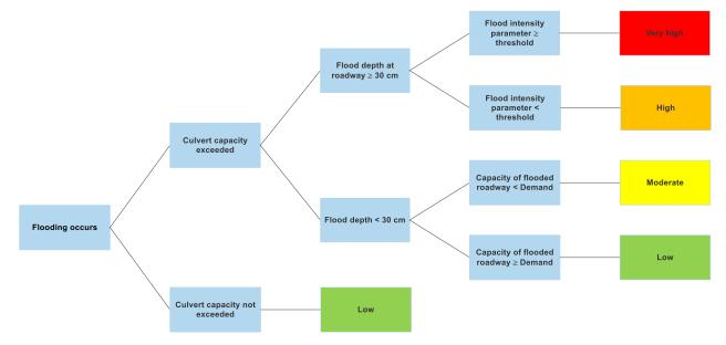
Figure 21: An example of an event tree for assessment of probability of different consequence classes for the flooding hazard
