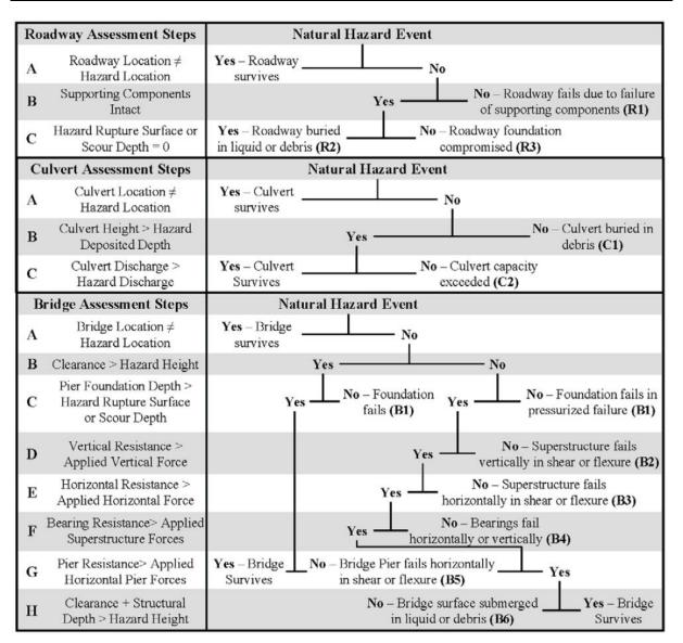
Figure 9: Structured component failure mode assessment approach
