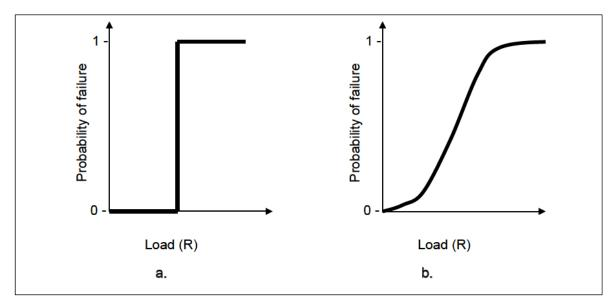
**Figure 6:** A conceptual fragility curve: (a) step function for very well understood or brittle systems; (b) an S-shaped function for poorly understood or elastic systems (USACE, 2010)
