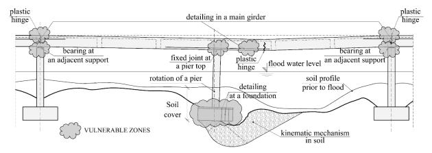
Figure 16: An example of a failure mode due to local scour at a pier - multiple-span RC girder bridge and its vulnerable zones - adapted from Tanasic & Hajdin, 2017
