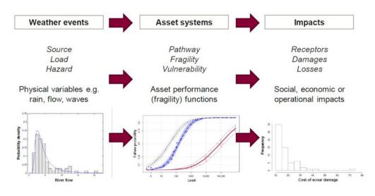
Figure 2: Conceptual risk model (Lamb et al.; 2017). The lower figure row applies to bridge failure from scour
