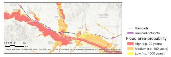
**Figure 20:** Exposure of railway track to floods for different flood return periods (20-years, 100years and 1000-years). The exposed parts of the railway are indicated with pink ellipses. (Source: *Ministerio para la Transición Ecológica, https://www.miteco.gob.es/es/agua/temas/gestion-de-losriesgos-de-inundacion/mapa-peligrosidad-riesgo-inundacion/*)
