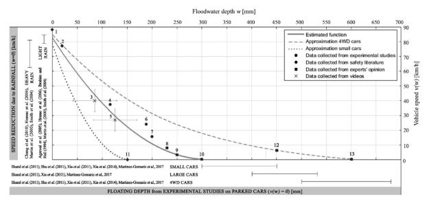
Figure 12: Depth-disruption function relating flood depth on a road with vehicle speed (Pregnolato et al. 2017)
