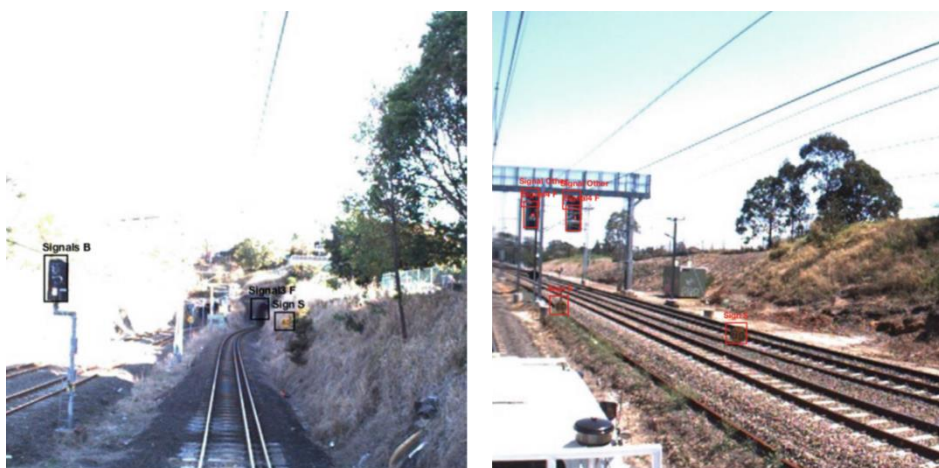
Figure 9: Signalization. Karagiannis, Olsen and Pedersen (2020) implemented a R-CNN for sign detection using RGB images
